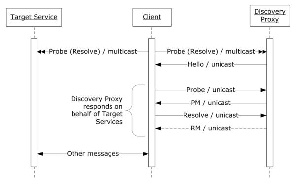
Figure 4: Discovery Proxy message exchanges.
